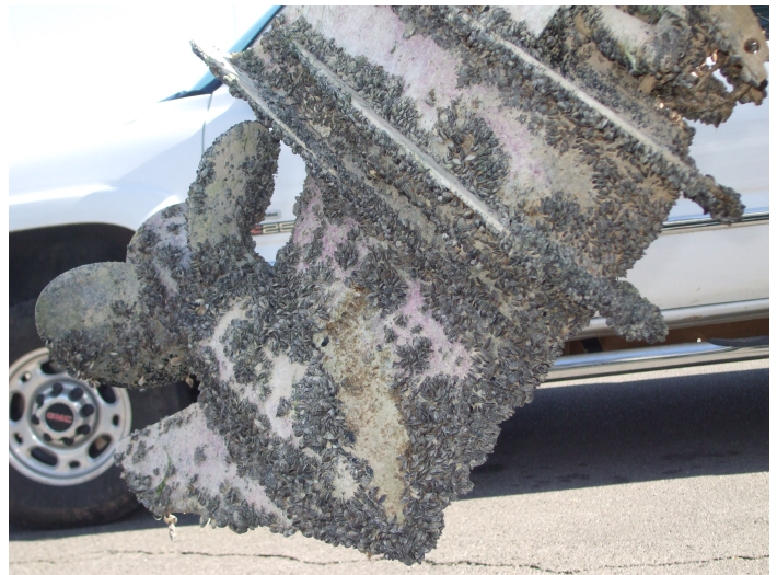
Quagga mussels can readily clog up a boat engine's cooling system to where the cooling does not function properly and the engine burns up.
