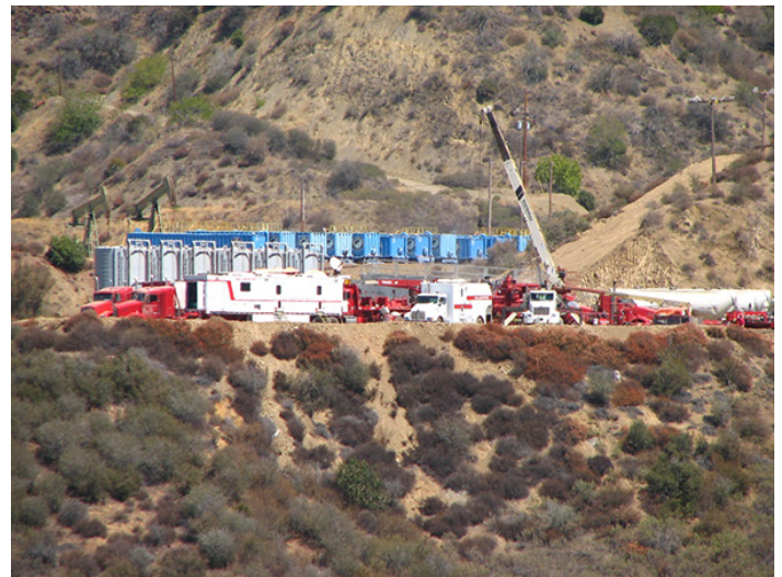
A Seneca oil well in the Sespe Oil Field in the process of fracking in 2013. The containers are full of fracking fluids.
